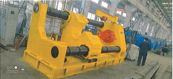
This machine is suitable for the disassembly and assembly of large wheel and axle components in industries such as railways, mines, chemicals, and steel production.
